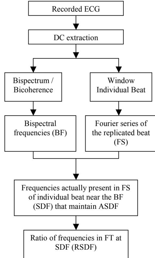
**Figure 1. Block diagram of the Frequency Detection procedure**
