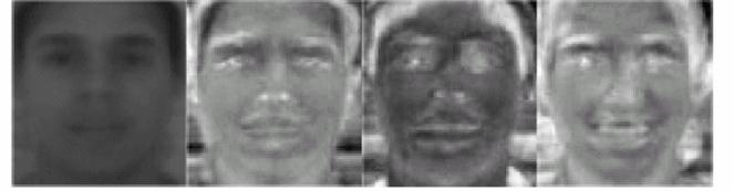
**Fig.3 Typical set of eigenfaces as used for face recognition. Leftmost image is average face.**
